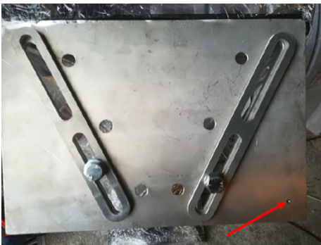
6 mm threaded hole - for grounding
