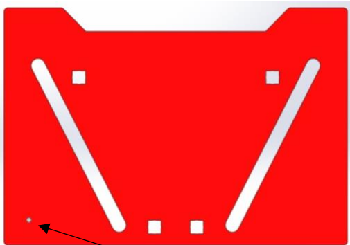
6mm threaded hole - for grounding
